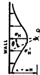
SECTION - - - PRESSURES FROM POINT LOAD Q_p (BOUSSINESQ EQUATION MODIFIED BY EXPERIMENT)
